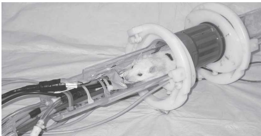
Figure 3 A 250-g rat prepared for imaging in a 2-T system using a 6-cm diameter birdcage coil. The animal is lying on a Plexiglas cradle and is anesthetized with isoflurane delivered by mechanical ventilation. The hoses to the left are for ventilation gases and the black cables carry signals from ECG electrodes on the foot pads, airway pressure transducer on the breathing valve attached to the endotracheal tube, and body temperature from a thermistor in the rectum. The lower cable connects the coil to the MR scanner.
