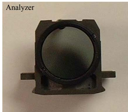
Figure 3. Analyzer cube.
