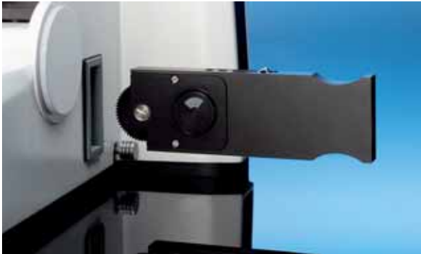
The Dodt Contrast slider is positioned in a conjugate plane to the aperture diaphragm...
