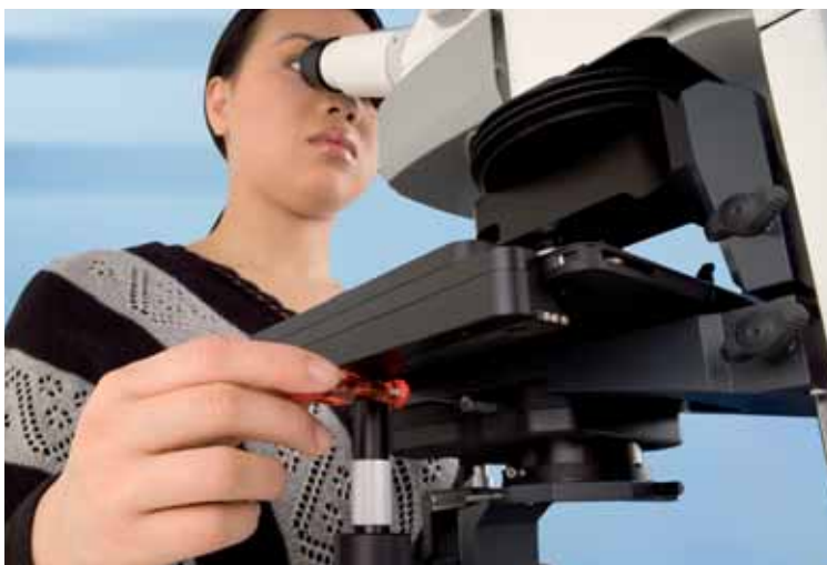
New standards even in simple contrasting: the segment diaphragm integrated in the condenser for oblique illumination can be turned through 360° and thus optimally adapted to the specimen structures orientation.
