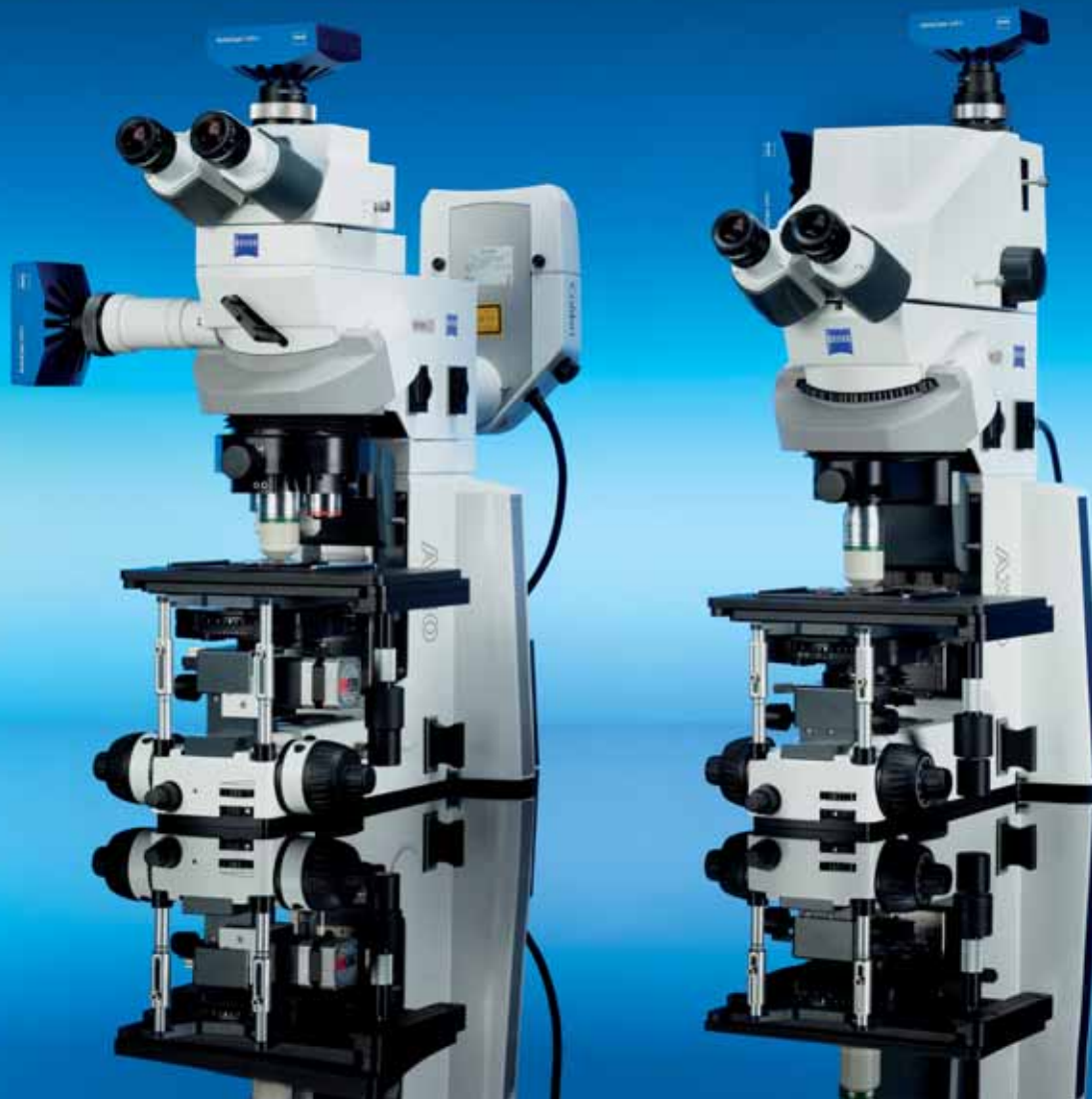
Axiolux Examiner in two of the three possible dual camera configurations.
