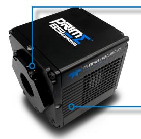
Backside Illuminated Sensor >95% peak QE 45,000e- full well 6.5 x 6.5µm pixels 18.8mm diagonal
