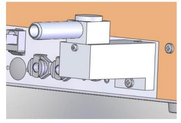
Figure 7-17. Rotating vacuum spigot
