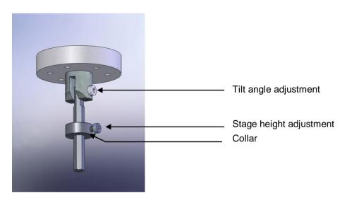
Figure 7-14. Adjustable tilting stage
