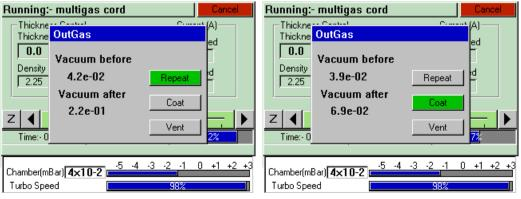
Figure 5-10. Prompts to repeat the outgas procedure (left) and proceed with coating (right)
