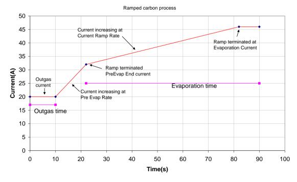
Figure 5-7. Ramped Profile with default parameters
