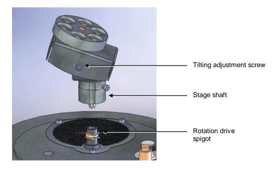
Figure 7-11. Rotacota stage
