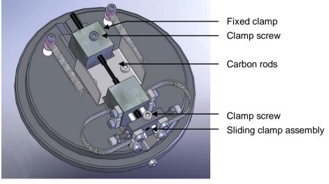
Figure 7-3. Carbon Rod Insert
