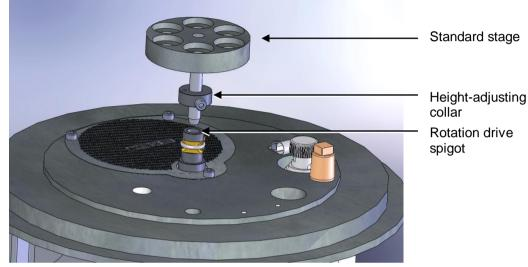
Figure 2-4. Fitting the standard stage
