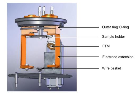
Figure 7-8. Metal evaporation insert adapted for upwards evaporation
