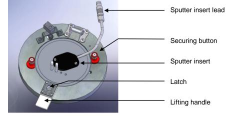
Figure 7-1. Top view of the sputter insert
