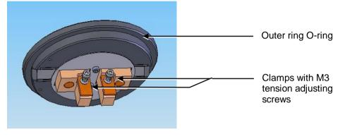
Figure 7-6. Carbon fibre insert
