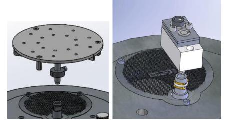
Figure 7-13. Large (102mm) Sample Stage and gearbox
