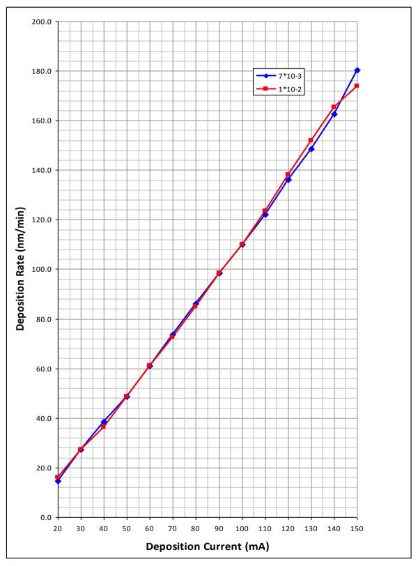
Figure 9-3. Sputtering Deposition Rate using Silver
