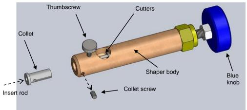
Figure 7-5. Carbon Rod Shaper (S8650/S8651))
