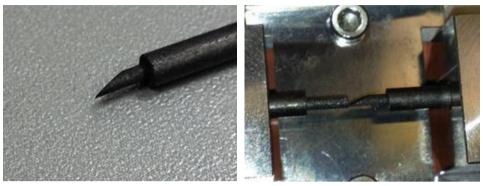
Figure 5-6. (I) A finished wedge-shaped rod; and (r) in position with plain rod
